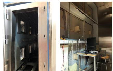
► Fig. 2: View of the two rooms of the Climate Simulator: the cold room on the left hand side, the cold room with solar simulator, on the right hand the warm room.
