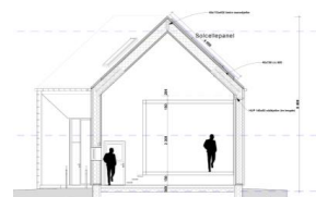
► Fig. 3: Vertical section of the ZEB Test Cells Laboratory with one test cell and one guarded volume.
