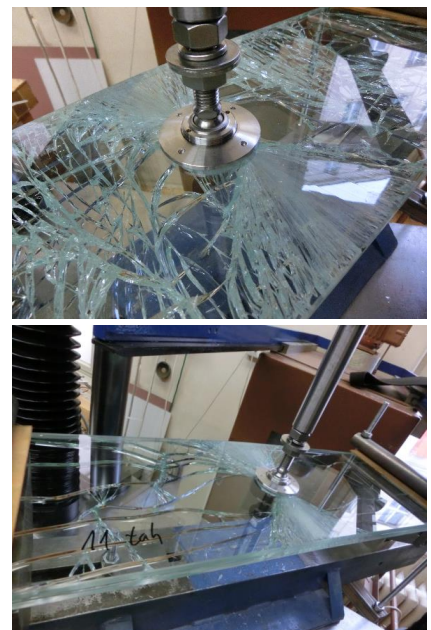
► Fig. 3: Non-standard connection tests of the façade glass panel performed at Klokner Institute, CTU in Prague
