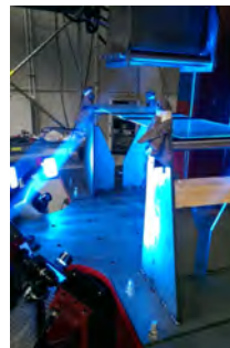
Left: Four-point-bending-test setup in high-speed testing machine. Right: Untempered float glass specimen in breakage phase during high-speed test monitored with high-speed camera in 30.000 fps mode.
